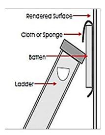
**N.B.:** Where possible please **do not lean** bikes, ladders – anything in fact – directly on to the walls of the house as it may damage the new system and render – which can make the insulation **ineffective**. Please be careful when taking out your bins too because any damage to the render, and / or insulation can have an impact.
