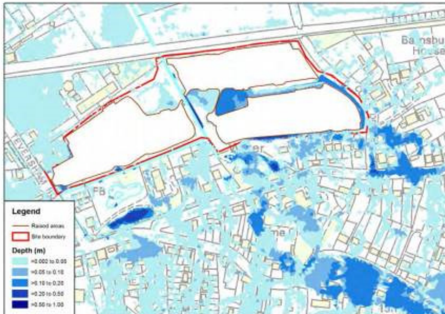
Figure 4.5: Surface water flood depths for the 1 in 30 year rainfall with the development in place
