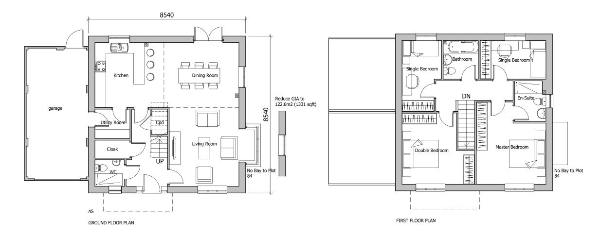
Note: Window positions and sizes may vary slightly dependent on house type character area location (internal layout is constant). This floor plan reflects the Village Lane character area variant. Please refer to general arrangement elevation drawings (P-13 series) for each character area.
