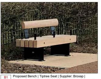
Proposed Bench | Tiptree Seat | Supplier: Broxap | Product Code: BX14 4030-BP | Galvanized steel legs with treated softwood | Finish: Black powder coated for metal members & arm rests| Fixing: Root fixed as per manufacturer's specifications
