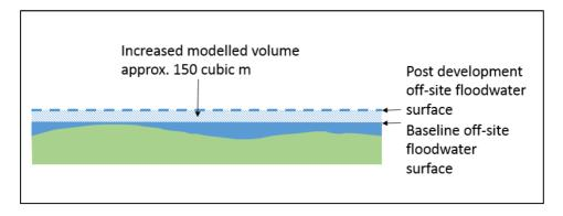
Illustration of the compensatory flood storage volume provided by the scheme.
