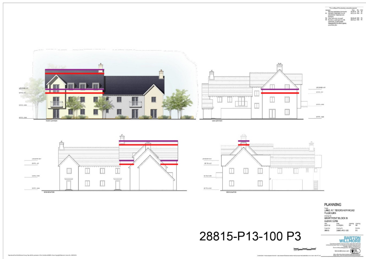
Fig 2.3.2 block B 28815-P13-100-P3 – red line = parameters height, purple =proposed height
