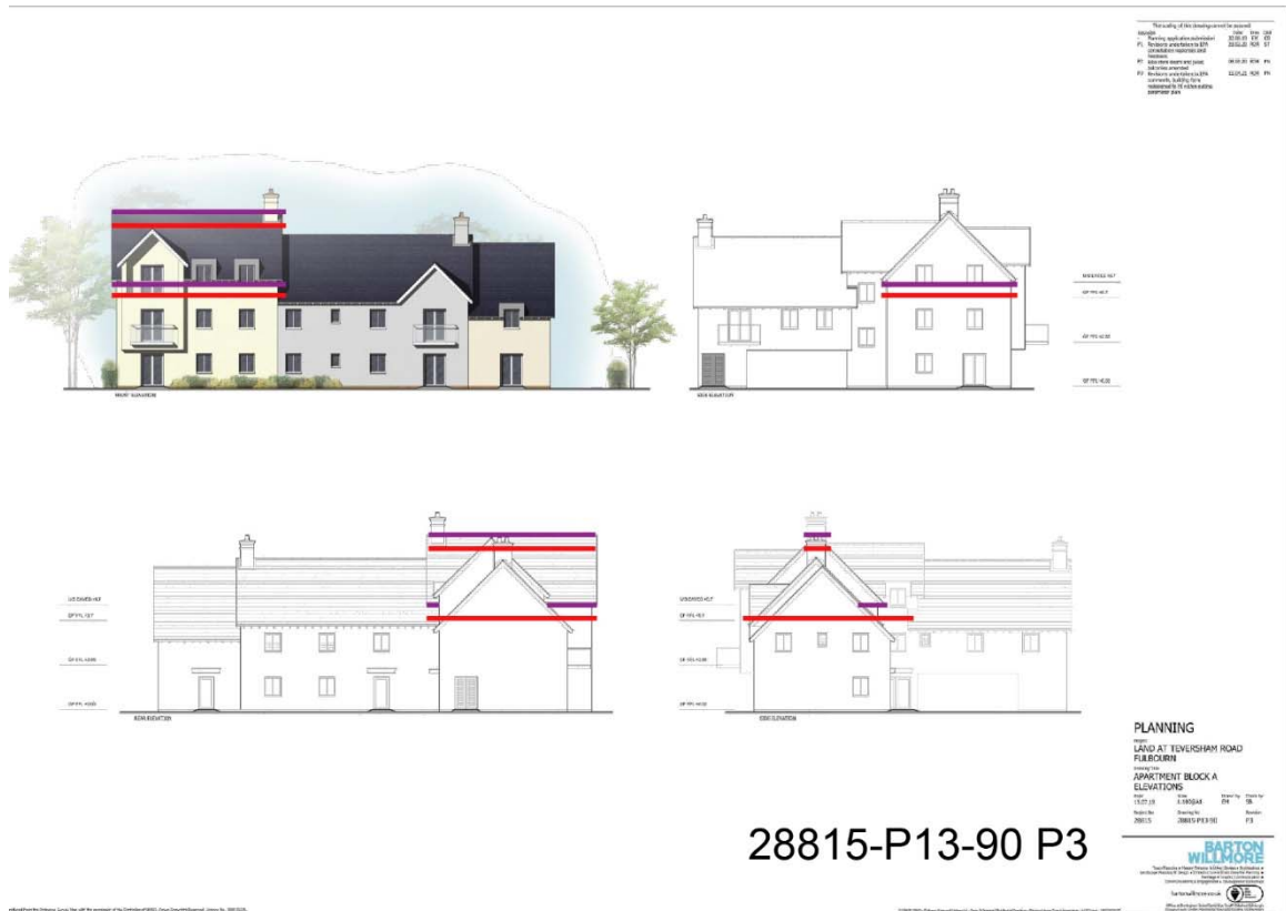
Fig 2.3.1 block A 28815-P13-90-P3 – red line = parameters height, purple =proposed height
