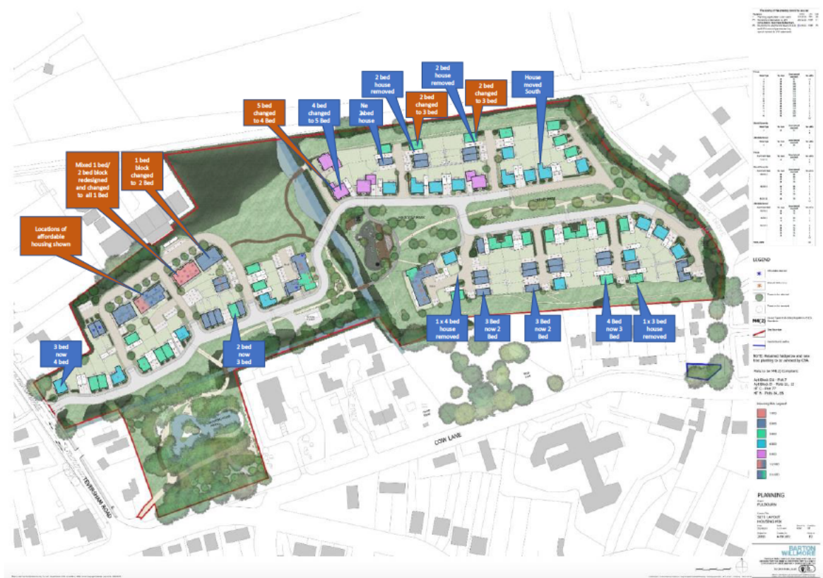
11. Figure 14: Final Housing Mix Layout Rev P2 (drawing dated 15.04.21) annotated with changes between Revs P0 and P1 in brown, and changes between Revs P1 and P2 in blue. See figures 15, 16, and 17 for 'easier-to-read' zoom views of each platform.
