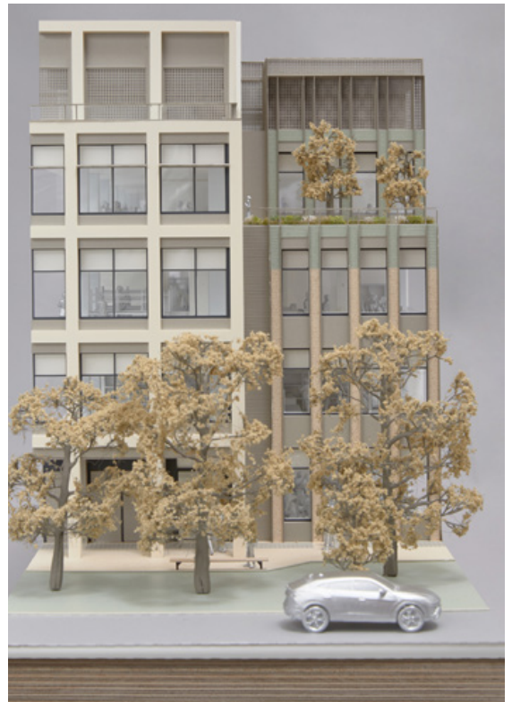
Fig. 32 Sectional bay model of 1&3 Station Row, exploring articulation of the eastern edge in detail and materiality.
