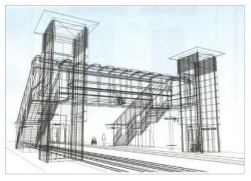
Figure 21 - AFA footbridge with lifts and stairs, 3D impression (extract from CoP)
