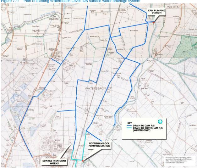
Plan of existing Waterbeach Level IDB surface water drainage system Figure 7.1:
