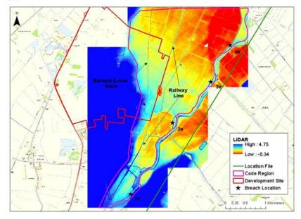
Figure F.2: Revised TUFLOW model extent and updated LiDAR topography data
