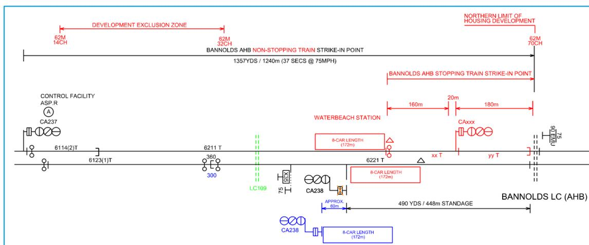
Figure 7 - Northern location station and signals configuration
