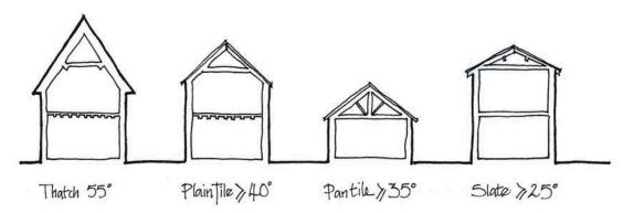
Diagram illustrating different roof pitches for different materials
