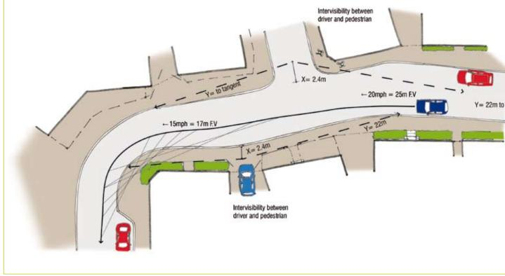
Fig:7.2 Visibility at junction Assessing vehicle speeds and visibility
